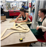
Step 1 CNC the ply wooden frame
