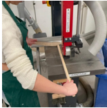
Step 2 Cutting timber dowels
