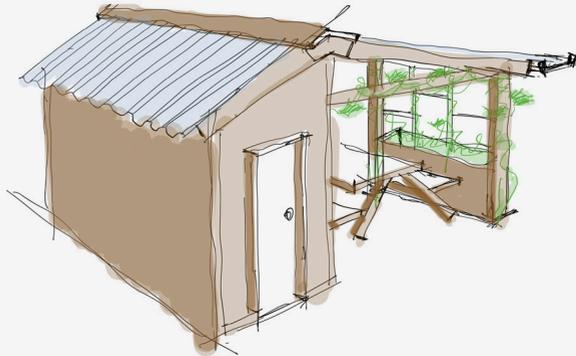
The next few days the team would construct a timber window frame for a recycled window, build a custom door, add an air gap for water drainage. Simultaneously the team would start constructing the green roof and fit the solar panel on top. This roof was not fitted in the Boiler House but would be finished on site. A waterproof membrane will be installed, as to not cause any tears when moving the flat-packed walls. Finally we cladded the walls and dismantled for flat packing.
